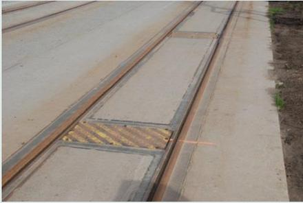
The WORM system (Wheel Out of Roundness Monitoring) is specifically developed for the detection of flats and out of roundness of wheels on heavy rail and light rail vehicles.
