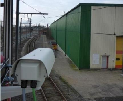
The PANTOCAM system is specifically developed for the measurement of wear on pantographs and the detection of defects and damage on current collectors of heavy and light rail vehicles.
